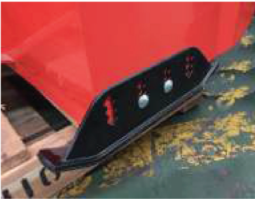
Image 1: Assembled Skid Shoe.
