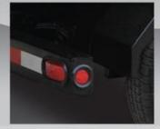
Rubber boots serve a dual purpose - to provide shock absorption protecting lights from impact time after time and to resist moisture.
