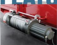
The big 12V Electric winch handles the job at hand. The free-spooling clutch gets you hooked up to deck or bin fast so you can get under way.
