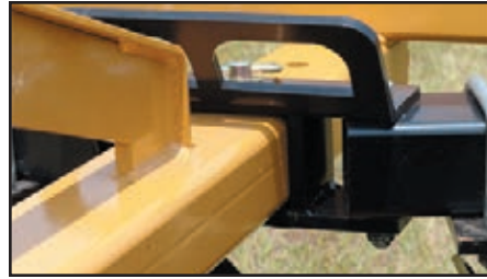
Easy-to-grasp handle for simple gang adjustment
