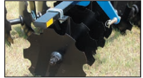
Notched discs for maximum cutting action
