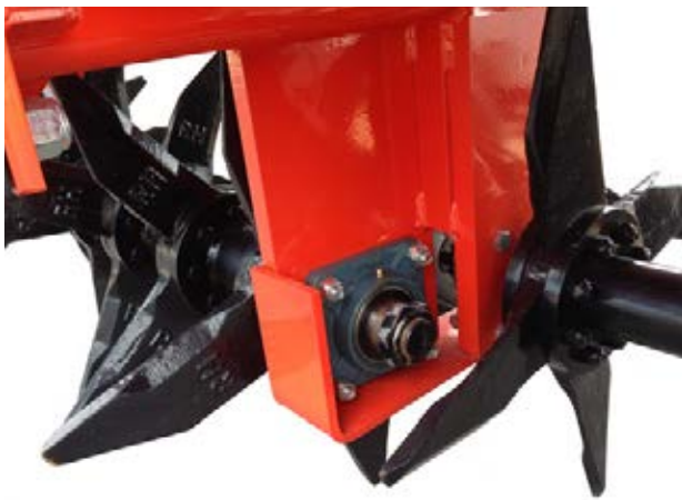
Heavy duty bearing hangers support the twisted shank rotors
