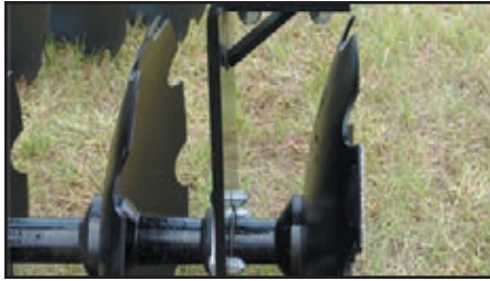
Bearing hangers reinforced with gussets
