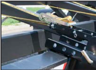
Two fully adjustable ratcheting straps for securing all brands of heads
