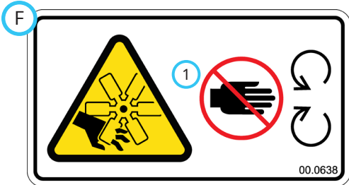
1. Severing of fingers or hand - engine fan. Stay away from moving parts.
