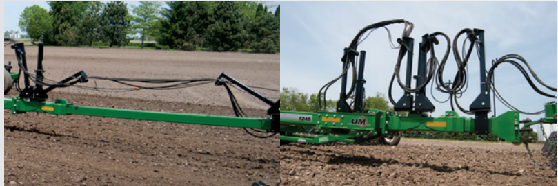
Hydraulically retractable tongue
