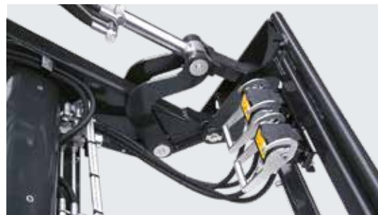
For even quicker hydraulic tube connection, the Tool-Fix for tool connection is available.
