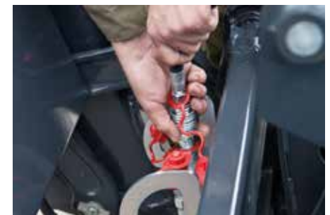
3 Couple the hydraulic connection
