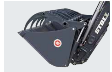
2 Roll back the tool – the locking mechanism will engage automatically
