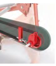
The elastic drive, which uses a V-belt and flanged pulleys, always transfers the power reliably by means of an automatic tensioner and protects the mower components from
