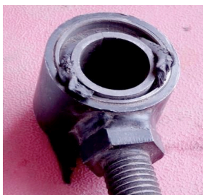
Old/Worn Bushing System
