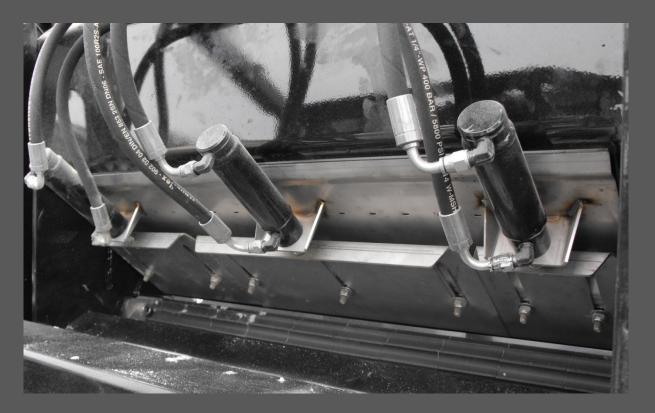
5 sections can be shut with swath control (GPS) or manually
