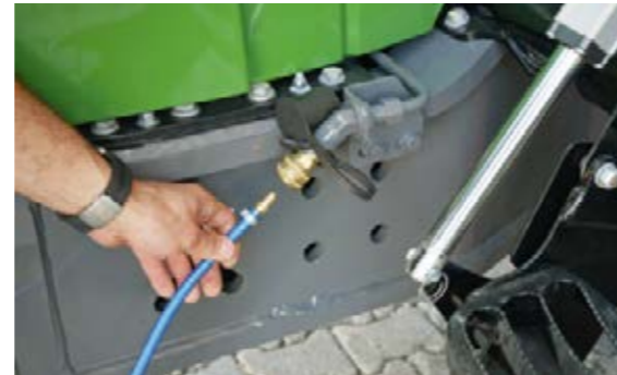
There is a compressed air connection at the machine front to blow out the air from the radiator.
