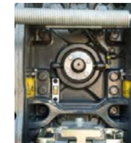
Select between two PTO speeds: 1000 and 1000E.
