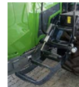
You can climb into the spacious cab via a ladder that can be folded up and down automatically.
