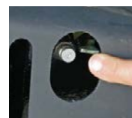
□ The pressure for pre-tensioning the rolling track can be comfortably adjusted from the side by means of a connection.
