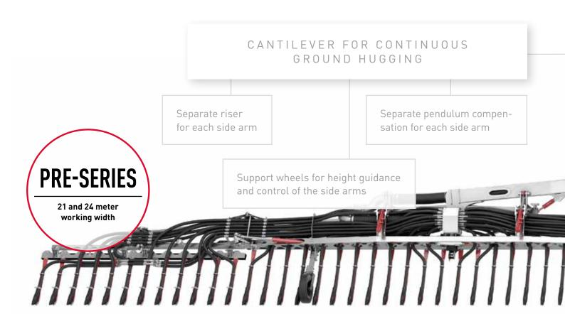
Tidy appearance, as all cables are integrated directly in the cantilever
