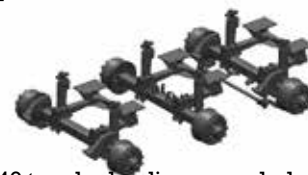
40 tons hydraulic suspended forced steered tridem
