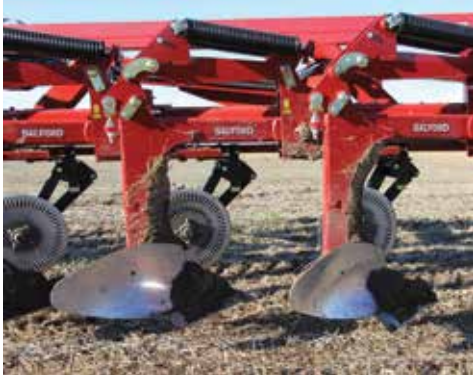
Superior shank geometry and construction provides the durability to handle almost 4000 lbs of trip pressure.
