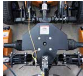
Transport Lock Quick Release Easily pull the rope to release transport lock.
