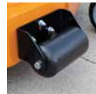
Optional Front and Rear Rollers Anti-scalp protection for uneven terrain.
