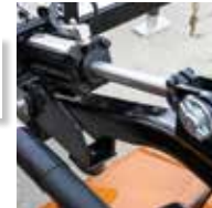
Hydraulic Cylinders Rugged, single-acting hydraulic cylinders fold the mower for transport.
