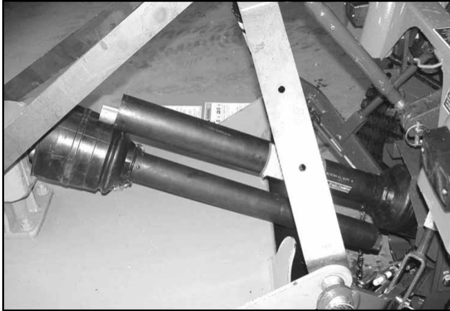
Figure 4. Drive Halves Placed Parallel
