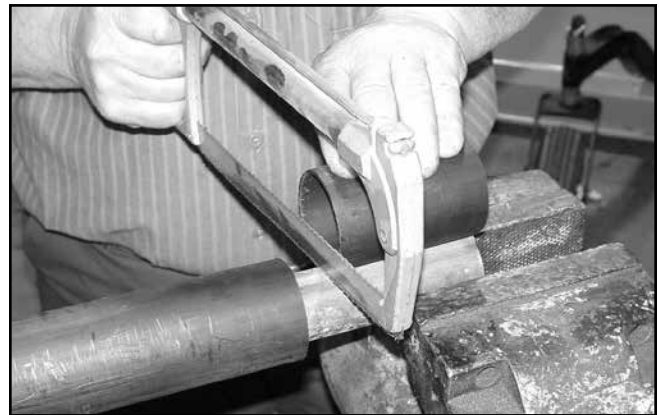
Figure 7. Cut Shaft to Length
