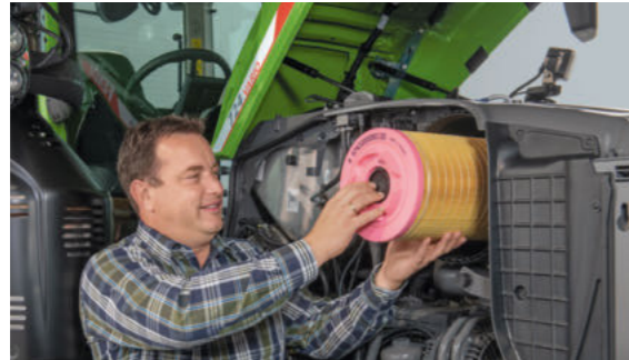
A swing-up bonnet and removable side panels provide excellent access to the engine compartment. This means you can quickly and easily remove the air filter.
