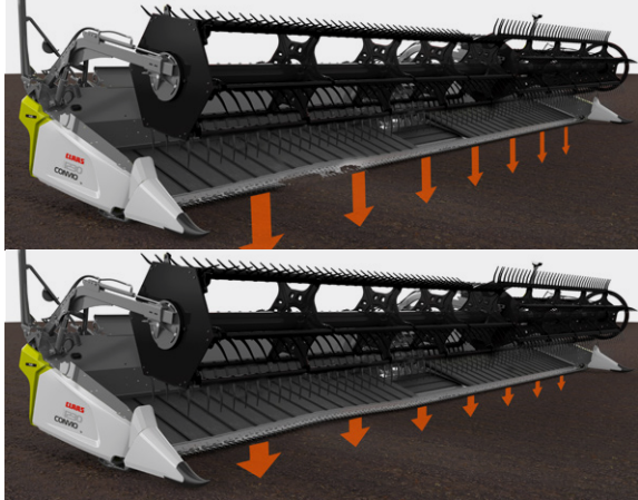
ACTIVE FLOAT allows ground pressure to be adjusted for the cab
