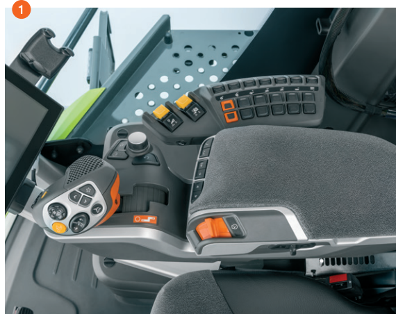
Reversing is possible with CMOTION (1) or toggle switch (2)
