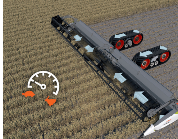
AUTOMATIC BELT SPEED matches belt speed to combine speed
