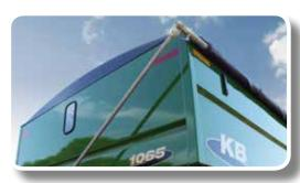
Weatherguard roll-over tarp to protect grain from adverse weather conditions
