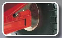
Heavy-duty bolt-on spindles allow for easy addition of scales
