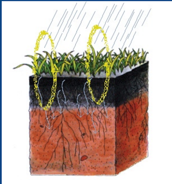
SMART-TILL®'s tines fracture soil more than 8" deep, allowing air (yellow) to be released and water (blue) to be absorbed more readily for healthier soil.
