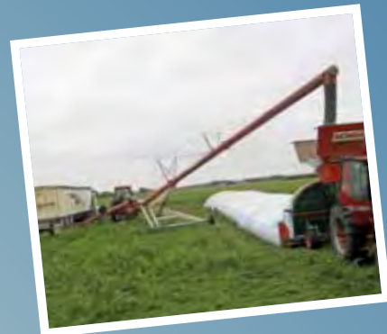
Aids grain bagger positioning, Auger-Steer also enables the auger spout to sway left and right making lining up even easier
