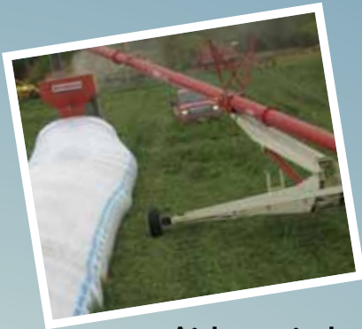
Aids grain bagger positioning, Auger-Steer also enables the auger spout to sway left and right making lining up even easier
