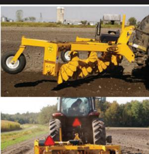
The WD-6 and WD-10B rock rakes are made to move rocks and roots into windrows making them easier to collect.
