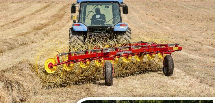
The new range of TR-S in-line trailed wheel rakes stands out from the traditional earlier range for its smaller transport dimensions and for being extremely easy to use and to adjust while working. The machine can be moved from the transport to the working position and back to the transport position from the tractor, using the hydraulic system. The machine's sturdy design provides excellent performance both in terms of quantity and quality.
