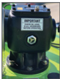
Convenient oil level site glass on gearboxes
