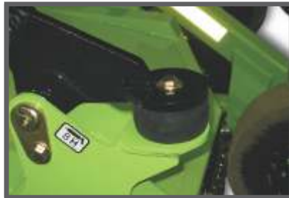
Self Adjusting Forward Mounted Slip Clutches
