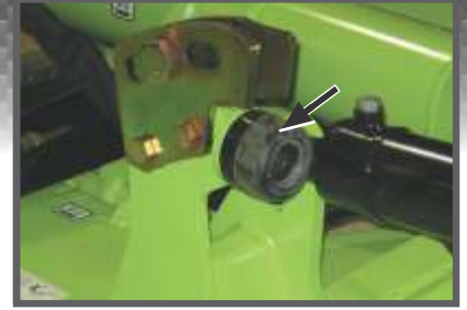
Wing Lift lock up with rubber stopper
