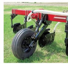
Both sizes feature adjustable down force and 7.60 x 15 adjustable gauge wheels.
