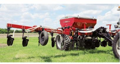
The Hiniker 6000 Side-dress Applicator is available in both 30- and 40-ft widths with a 7-ton, #409 painted stainless hopper. Both 30- and 40-ft sizes feature automatic 8-degree wing tilt for additional crop clearance on end rows.
