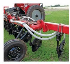
Toolbar underframe clearance is a generous 30 inches in working position. The 16-row model may be used as a 12-row applicator with outer wings folded.
