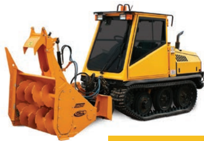
S-250 HD snow blower Hydraulic drive system.
