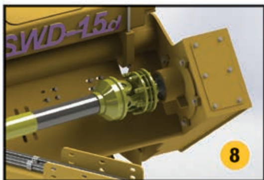
Multiple disc slip clutch.
