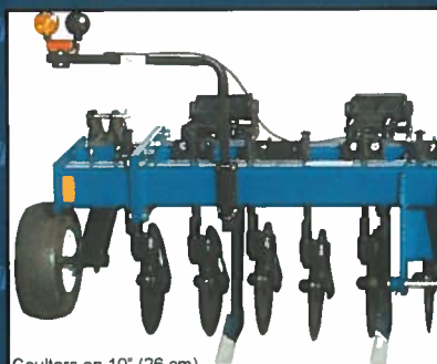
Optional StalkSizer slices stalks and improves tough residue flow
