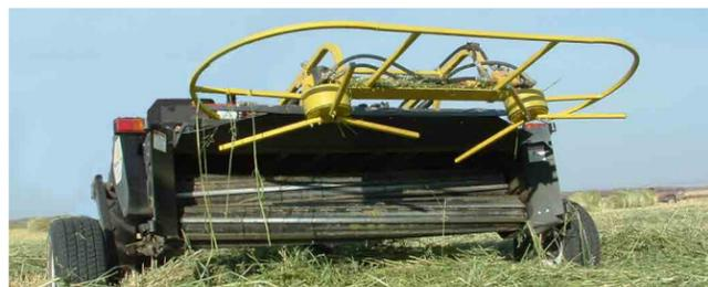
In the rare case that you plug the machine, the ReCon's rollers open hydraulically from the cab to un-plug the machine in seconds
