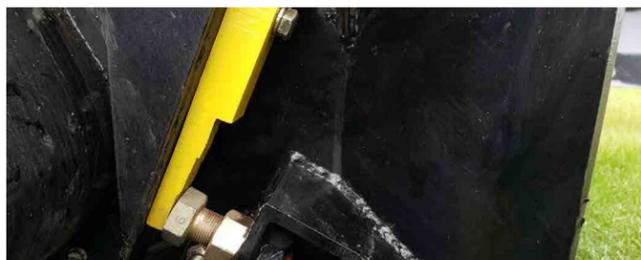
Quick set sliders allow you to adjust and optimize roller clearance for various crop conditions
