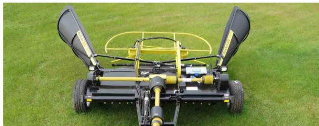
Ensuring ultimate reliability with minimal maintenance, crushing rollers are driven independently with high strength 80 chain in a sealed oil tight case
