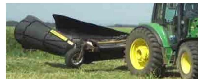
ReCon 400 jumps pivot irrigation tracks well because the ReCon tires have a fraction of the weight, and larger rear tractor tires and able to jump the pivot tracks better
