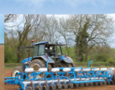
Mechanical planter for pelleted sugarbeet MECA V4
