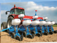
Multi-purpose pneumatic NG Plus 4 planter with discs
