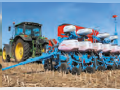
Special pneumatic « low-till » planter Monoshox NX M with discs
