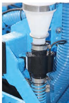
Sensor for fertilizer passage control
