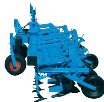
12-row front-mounted cultivator with «inversed units» with 45cm inter row spacings
