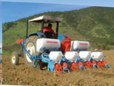
Multi-purpose pneumatic planter with NC shoes
