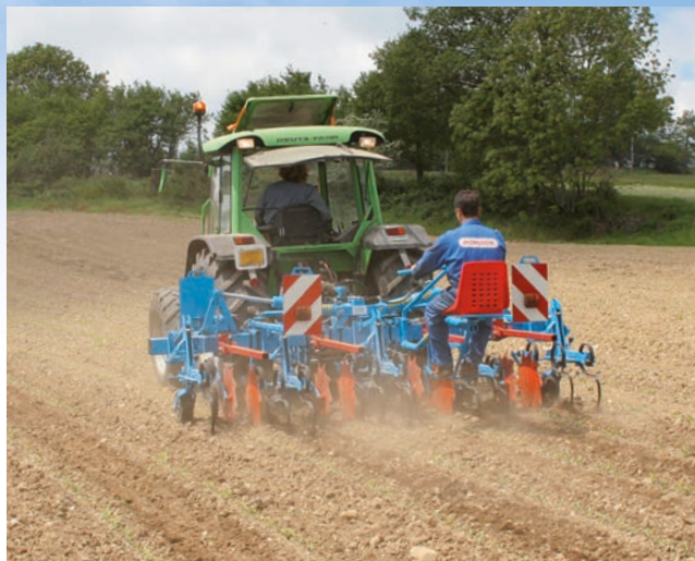
The steering wheels (1), orientated by the steering bar (2), can be adjusted in height (3).
