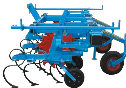
Standard 4-row front-mounted cultivator with 75cm inter row spacings
