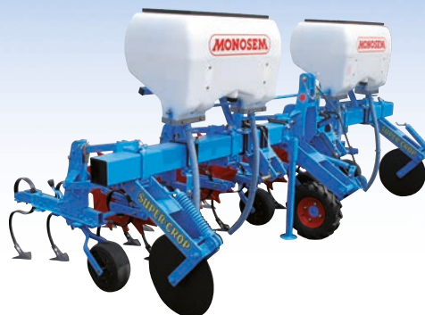
TIP 5" rigid cultivator – 4 rows at 75 cm inter row spacing
