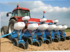
Multi-purpose pneumatic NG Plus 4 planter with discs
