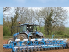
Mechanical planter for pelleted sugarbeet MECA V4
