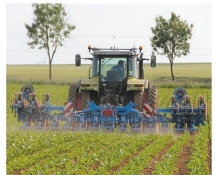
Partially folded, the «Wide Configuration» cultivator can also cultivate 8 rows in maize or 12 rows in sugar beet. This means only using one cultivator in fields planted with planters of different widths!
