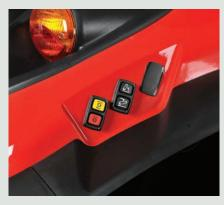
Push buttons in both rear fenders allow the operator to control the PTO and the rear 3-point hitch from the ground for convenience. (tractor must be properly equipped)
