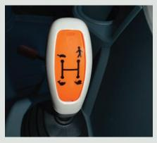
**X5.40** and **X5.50** models availble with factory creeper gear set. Located as a 4th position on the range lever, the creeper is ideal for special applications that require the tractor to operate at high RPM's with very low ground speed (0.24 mph / 0.39 kph)
