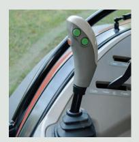
**X5.40** and **X5.50** models are available with 3-speed powershift option that gives operators the ability to quickly upshift and downshift through 3 power shift gears using 2 buttons integrated into the main transmission lever.
