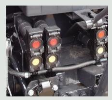
All X5 models feature an open center hydraulic system with 24.5 gpm flow. The dedicated pumps allow for 7.9 gpm (30 lpm) for steering and 16.6 gpm (63 lpm) for implements. **X5.30** models come with 2 rear remote valves, while the **X5.40** and **X5.50** have 3 rear valves.
