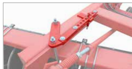
ADJUSTABLE GANG ANGLE Gang angles are pin-stop adjustable from 16 degrees to 25 degrees. Ratchet-jack on rear gang allows side-to-side gang adjustment to fine-tune performance.
