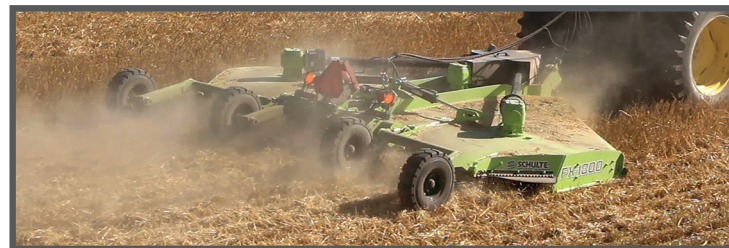
Optional Fixed Knife system. Outboard blade rotation keeps material from balling up under the deck
