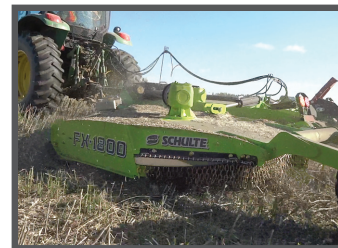
Optional Fixed Knife system. Outboard blade rotation keeps material from balling up under the deck
