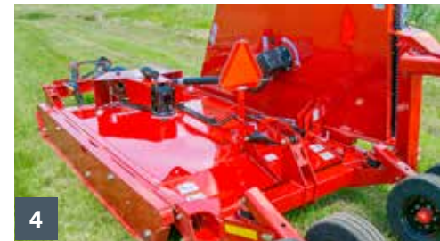
[1] 250 splitter with 190 HP Gearbox [2] Independent wheel assembly suspension [3] Industry leading blade tip speeds [4] Smooth top deck.
