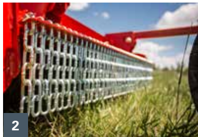
[1] 120 and 90 HP gearbox [2] Standard chain shielding, stump jumper and replaceable front skids [3] 21 inch laminated solid rubber wheels [4] Flat top deck.
