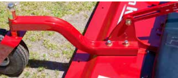
[1] Independent axle beams. [2] Pneumatic tires with puncture proof sealant are standard; solid rubber tires can be equipped as an option. [3] All models are quick hitch compatible.
