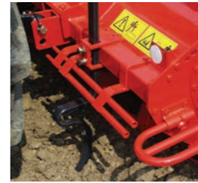
TRACK ERADICATORS Loosen the soil behind tractor wheels. Made up of four flexible tines adjustable in height and distance.
