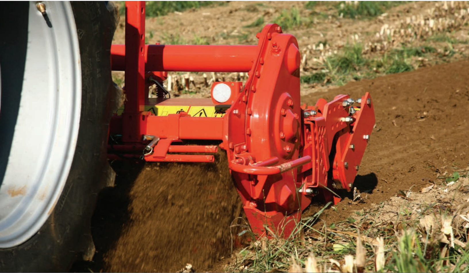
SIDE SEPARATING DISCS Avoid ridge formation between two passes and facilitate work in long plant residues. Easily adjustable by a pin.
