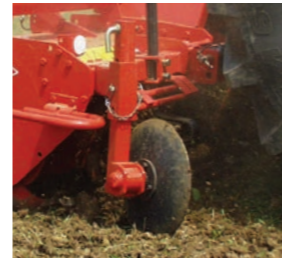
SIDE SEPARATING DISCS Avoid ridge formation between two passes and facilitate work in long plant residues. Easily adjustable by a pin.
