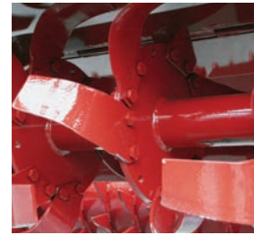
COUNTER FLANGES EL 92 power tillers can be fitted with counter flanges for reinforced blade hold in rocky conditions.
