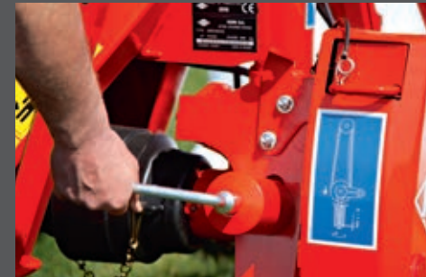
SEMI-AUTOMATIC BELT TENSION
