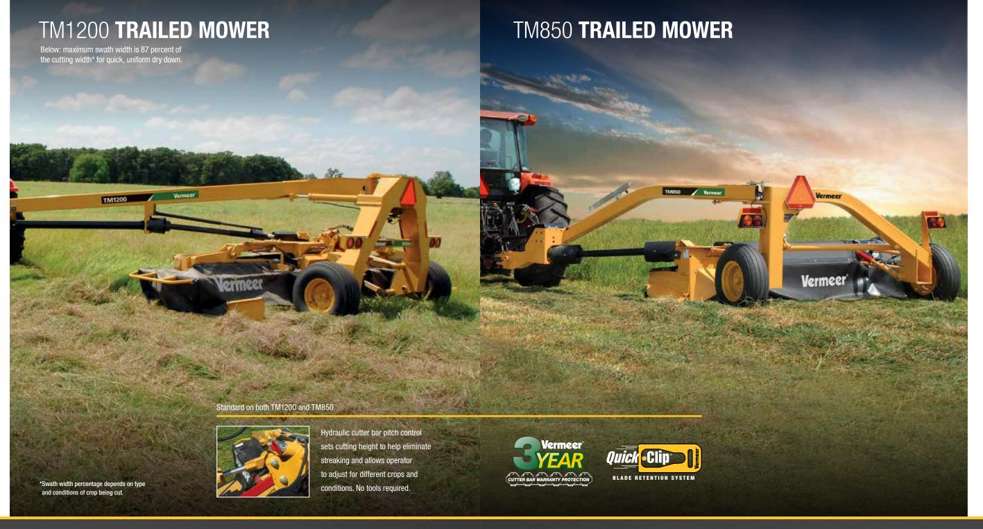
When you first see the TM850 trailed mower alongside other 10 ft (34 m) trailed mowers, you immediately understand why it's considered the real heavyweight in its class. Simply stated, this one's built to handle a regular diet of high-volume material, while maintaining a required low 60 hp (44.7 kW) tractor.
