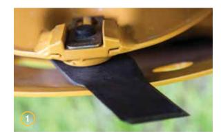
The Quick-Clip Blade Retention System allows the operator to quickly replace or reverse blades. Simply slide out the clip, reload the new blade, tap it in place with the provided tool and get back to mowing.
