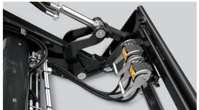
2 Tilt the implement – the locking mechanism engages automatically
