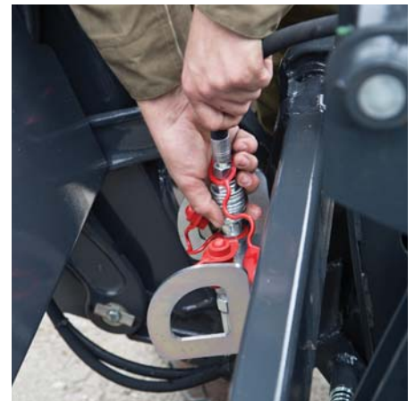
3 Coupling of the hydraulic connection
