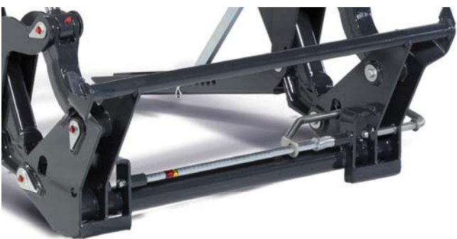
All implements with euro attachment fit in the euro quick-change frame.
