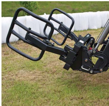
2 Tilt the implement – the locking mechanism engages automatically
