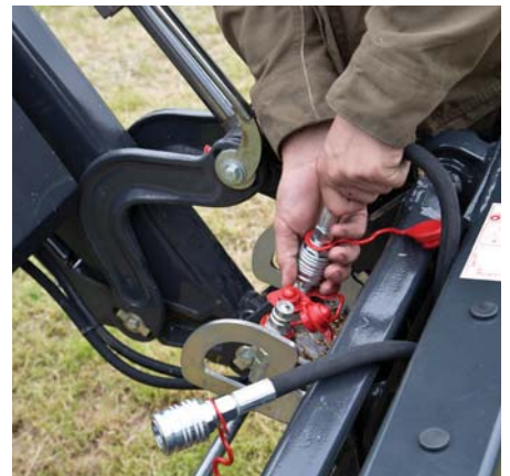
3 Plug in the hydraulic connection
