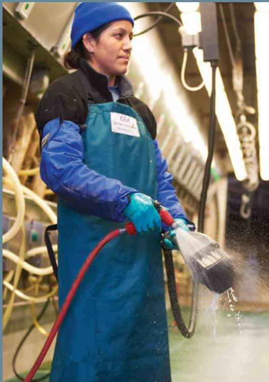
*The FutureCow® Prep System from GEA accomplishes multiple pre-milking procedures in one easy step. The system features a mechanical brush unit that gently washes, disinfects, stimulates and dries all in one visit to the cow. Cows receive superior stimulation and a consistent prep procedure, no matter who is milking. Dairy producers can potentially reduce labor costs and can certainly reduce operating costs by eliminating towels and laundry.*
