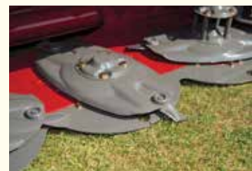
A low-profile, spur gear cutterbed that's thinner in design, means closer cutting.
