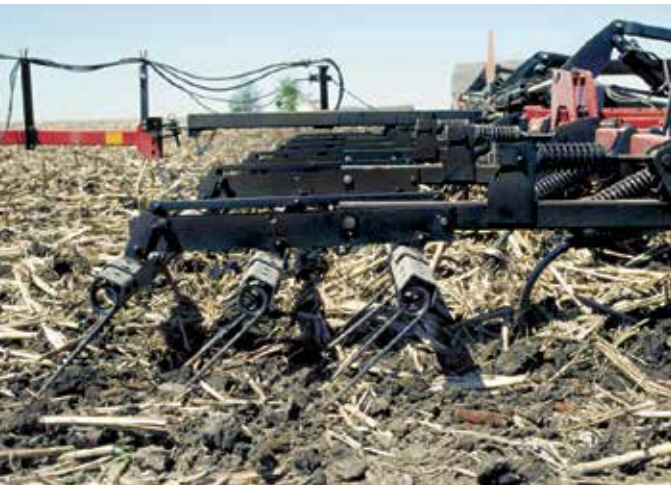
The Coil Tine Harrow has a 3-bar design and 15 in. (38 cm) rank for excellent residue flow and leveling. This harrow utilizes 16 in. (41 cm) long, 7/16 in. (11.1 mm) diameter double-coil tines with 2-1/2 in. (63.5 mm) effective spacing. Tines rotate to prevent damage when backing up.
