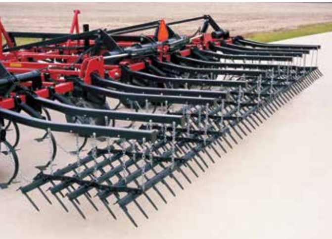
The Spike Tooth Harrow has a 5-bar design and 10 in. (254 mm) rank for excellent leveling and clod breakage. This harrow utilizes 11 in. (279 mm) long, 3/4 in. (19 mm) square width teeth with 1-1/2 in. (38 mm) effective spacing.
