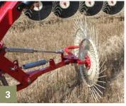
[1] The double frame pull bar and heavy main frame come together to make one of the heaviest rakes in the industry [2] Simple swath adjustment achieved with a bushing system; three preset widths available [3] Optional center mounted hydraulically operated wheel rake available for moving forage in the central zone. [4] Maximum transport width of 8'.
