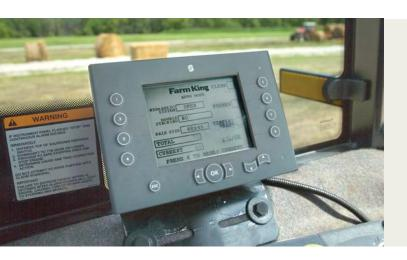
A hand-held control and a system monitor are responsible for programming and operating the Farm King 4480 Square Bale Carrier. The hand-held control activates the pickup arm and initializes the pickup sequence and operates the pusher and tilt deck.
