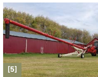
[1] Safety locking ball valve restricts hydraulic lines from losing pressure. [2] Load carrying tapered thrust bearing supports the weight of the flighting with auger in upright operating position. [3] Cleanout is simplified with an optional reverse kit and an underside access panel. [4] Durable 11 gauge flighting is used on every 10" and 13" model. [5] 11' to 15' transport height and standard road lighting kit. [6] Hydraulic Winch - An optional hydraulic winch easily lifts the hopper into place for transport. The lever and hydraulic valve are mounted to the main auger tube for easy access.
