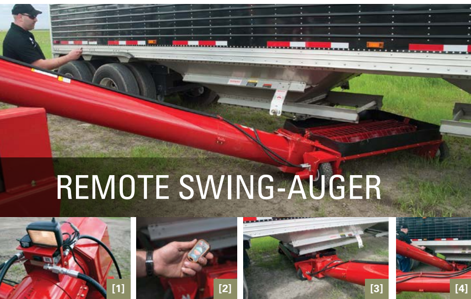
[1] Adjustable light kit for models 10"-14" (standard equipment on 16" augers) [2] Remote control [3] Self-leveling hopper [4] Remotely swing the hopper in place in seconds.
