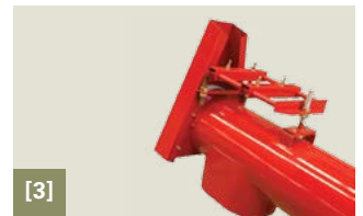
[1] Hopper [2] Hydraulic drive with variable speed control [3] Electric-drive models have an adjustable motor mount
