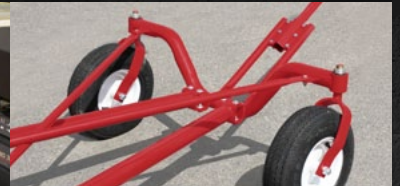
Narrow dolly frame wheels allow excellent maneuverability and raise completely for transport. These wheels easily fit between hopper bottom bin uprights for unloading convenience.
