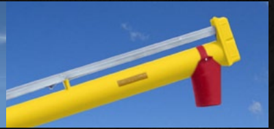
Bolt on downspout.
