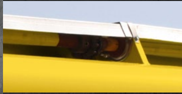
Chain coupler on driveshaft.
