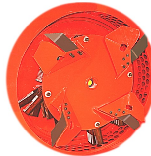
Knife system for high feed rate - use only with screen hole sizes greater than \frac{1}{2} " dia.
