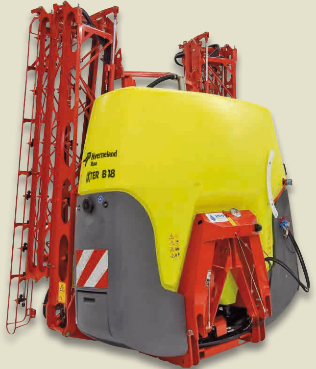
HC 18/20/21/24/27/28/30m vertical folding Steel-Liner booms
